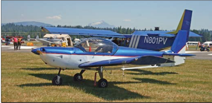
The CH 601 series has used a variety of engines. This example mounts a Corvair auto-engine conversion.
